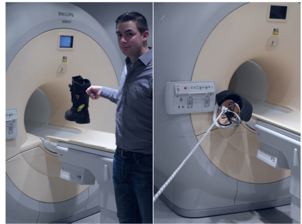
Figure 3. Testing of Boots and Helmet. The boot is floating freely due to the high force of attraction and the helmet needed to be secured by ropes.
