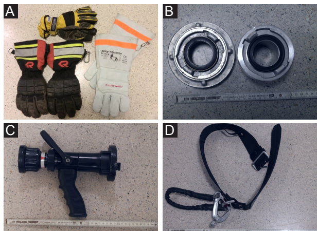
Figure 1. Examples of Selected Test-Items; (A) Gloves, (B) Firefighting house coupling and adapter piece B to C, (C) Fog nozzle and (D) Firefighting belt.
